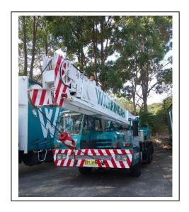
Underwent full restoration, and extensive rebuild in Nov 2013 (over \$360k spent) and body is as new condition. New Slew Ring and rebuilt hydraulics. Comes complete with full set chains, slings, timbers, along with 2 hooks, and is ready to operate
